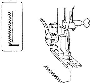
Set the pattern selector dial at “ $\begin{matrix} 4 \\ 2 \end{matrix}$ ”, sew 5 stitches of bartack and raise the needle from the fabric.
