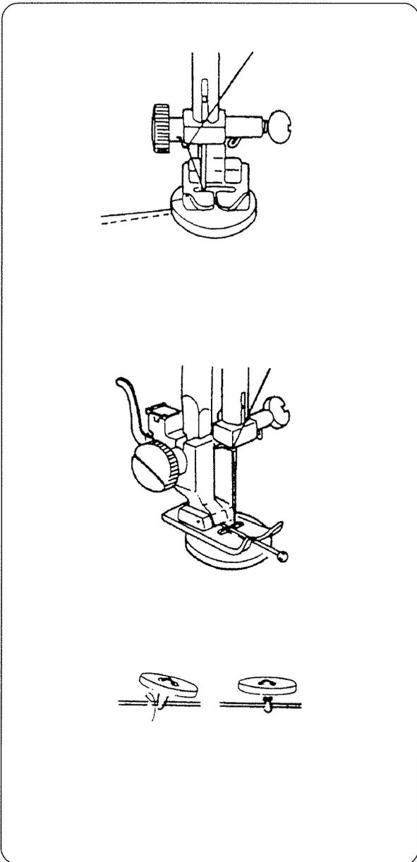
A pin can be placed on top of the foot to form a shank. Set the pattern selector at “ **B** ”.
