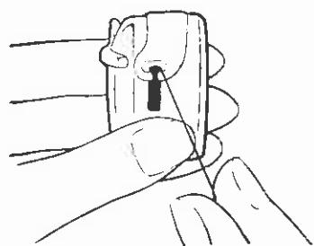
② Pull the thread into the bobbin case slot.
