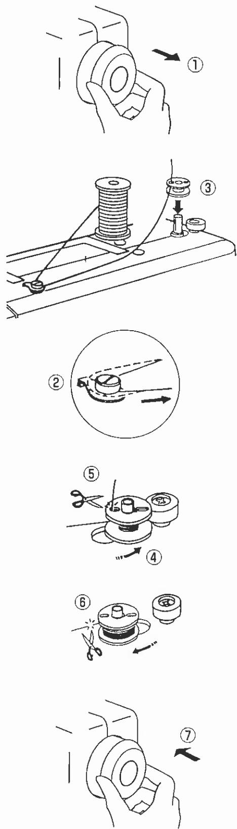
① Pull the handwheel out.
