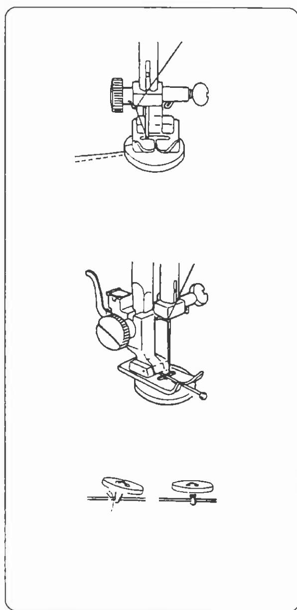
A pin can be placed on top of the foot to form a shank.
