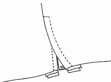
Pin or baste zipper tape to fabric and place it under the foot.
