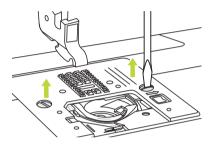
Remove the needle, presser foot and presser foot holder. Remove the screw holding the needle plate and remove the needle plate.
