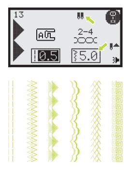
Press the twin needle button " . The LCD screen will display the twin needle icon " . and the machine automatically reduces the maximum width for twin needle sewing by 2mm.
