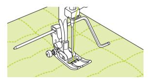
Sew the first row and move over the fabric to sew successive rows with the guide riding along the previous row of stitching.
