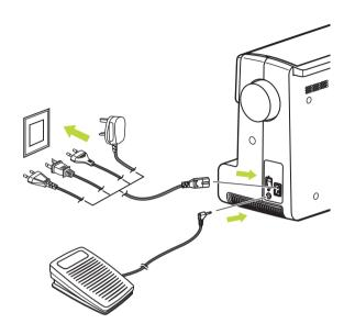
Before connecting the power supply, make sure that the voltage and frequency shown on the rating plate is conforming with your mains power.
