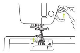
When sewing several layers or thick fabrics, the presser foot can be raised a second stage for easy positioning of the work.
