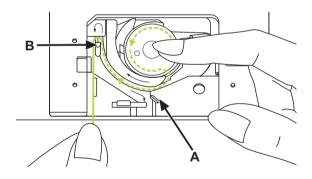
With a finger held gently on top of the bobbin. Draw the thread at the arrow markings into the stitch plate thread guide from (A) to (B).
