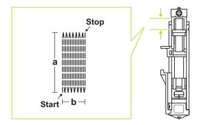
The size of one darn cycle is variable. However, the maximum stitch length is 2.6cm (1 inch) and the maximum stitch width is 7mm (9/32 inch).
