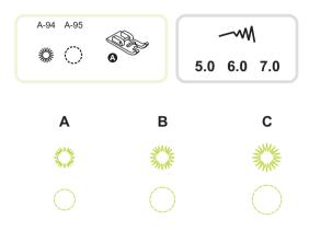
A-94 : Select for sewing eyelets on belts , etc A-95 : Select for sewing eyelets on belts , etc
