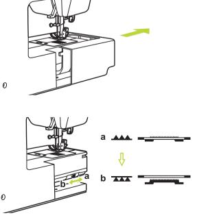
With the sewing table off the machine, the feed dog adjustment lever can be seen on the base in back of the sewing machine.
