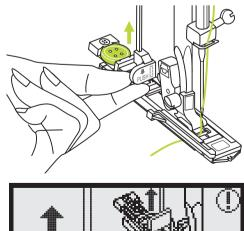
Raise the presser foot and cut thread. To sew over same buttonhole, raise the presser foot (will return to original position). After sewing the buttonhole stitch, raise the buttonhole lever until it stops.
