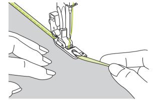
Lower the presser foot and start sewing slowly guiding the raw edge of the fabric in front of the hemmer foot evenly into the scroll of the foot.
