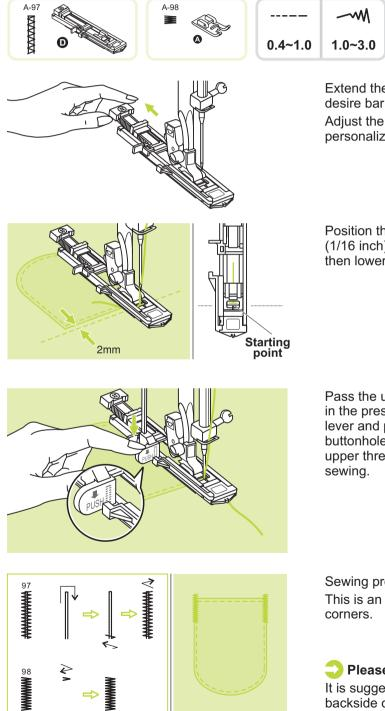
Extend the button holder plate and set to the desire bar tack length.
