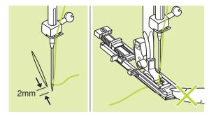
Position the fabric so that the needle is 2mm (1/16 inch) in front of the area to be darned, and then lower the presser foot lever.
