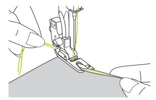
Insert the needle into the fold by rotating the handwheel toward you, and lower the presser foot. Sew several stitches and raise the presser foot.
