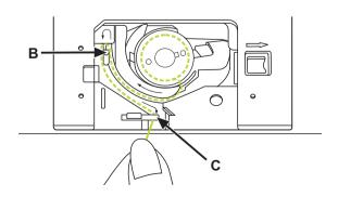
Pull the thread at the arrow markings into the stitch plate thread guide from (B) to (C). To cut off excess thread pull thread back over the cutting off blade at point (C). Close the bobbin cover plate.
