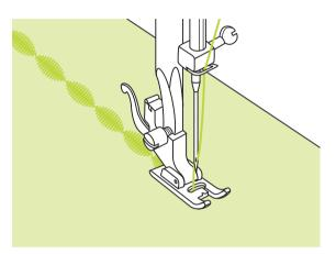
Use the satin stitch foot for satin stitching and sewing decorative stitches. This foot has a full indentation on the underside to allowed easy sewing over the thickness of the stitches form by closely spaced zigzag stitches, and even feeding of the fabric.
