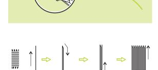
Darning stitches are sewn from the front of the presser foot to the back, as shown.
