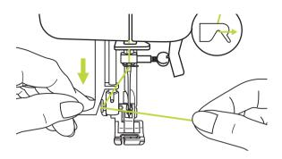
Raise the needle to its highest position and lower the presser foot.
