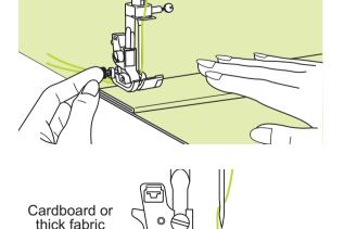
You also can place another piece of fabric with the same thickness at the back of the seam. Or support the presser foot while feeding by hand and sewing toward the folded side.
