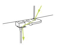
7. Pass the thread behind the flat, horizontal thread guide. Guide the thread through the wire loop.Pull the end of the thread through the needle from front to rear, and pull out about 10 cm of thread.Use the needle threader to thread the needle. (On the next page.)
