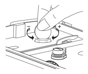
The presser foot pressure of the machine has been pre-set and requires no particular readjustment according to the type of fabric (light-or-heavy weight).
