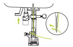
Hold the thread loosely and release the lever slowly. The hook will turn and pass the thread through the needle eye forming a loop. Pull the thread through the needle eye.
