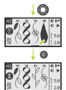
Press the desired pattern number or the arrow buttons to select desired pattern. (E.g. B group pattern 54)
