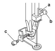
Remove the presser foot holder, and attach the embroidery foot to the presser foot holder bar. Press the embroidery foot on firmly from behind with your index finger and tighten the screw.
