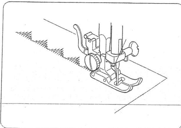
Sew a row of stitches and adjust the thread tension so the upper thread should appear on the reverse side of the fabric.
