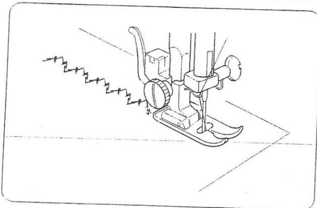
If forward and reverse feeds become unbalanced due to the type of fabric, adjust the balance by turning the stitch length dial as follows:
