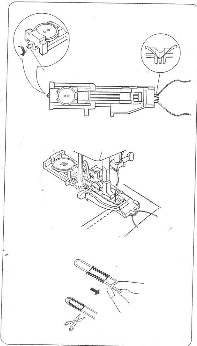
1. With the buttonhole foot raised, hook the cord on the cord spur at the back of the buttonhole foot.
