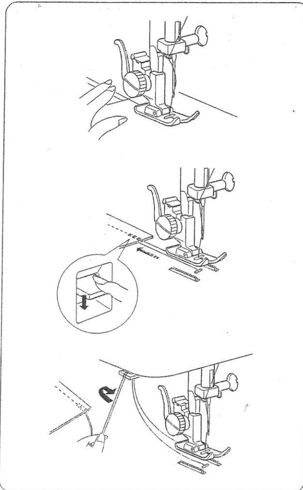
Raise the presser foot and position the fabric to a stitching guide line on the needle plate.
