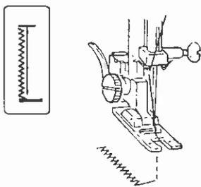
Set the pattern selector dial at “ 2 ”, sew 5 stitches of bartack and raise the needle from the fabric.
