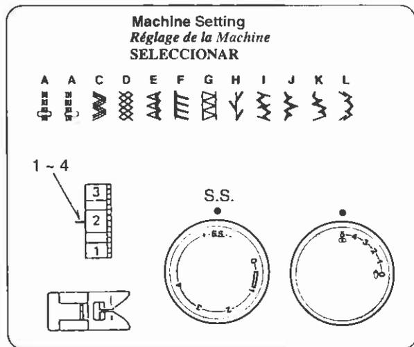
If forward and reverse feeds become unbalanced due to the type of fabric, restore the balance by turning the stitch length dial as follows:
