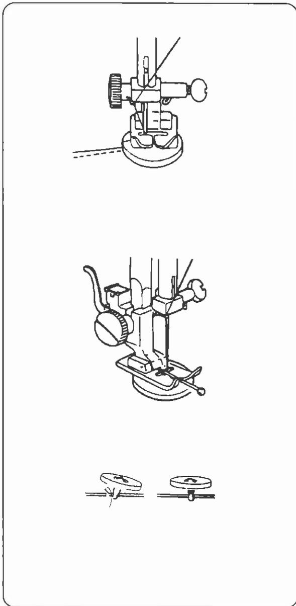
A pin can be placed on top of the foot to form a shank. Set the stitch width dial at "0".
