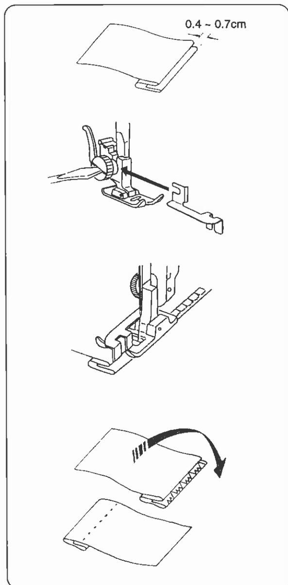
Raise the presser foot and place the fabric under the foot so that the soft fold rests against the wall of hem guide.
