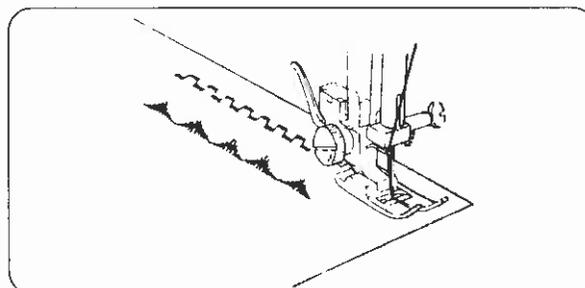
Sew a row of stitches and adjust the thread tension so the upper thread should appear on the reverse side of the fabric.
