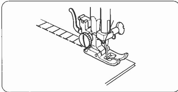
Overedge stitch will be done most successfully when the right side stitches of zigzag fall slightly off the edge of the fabrics.
