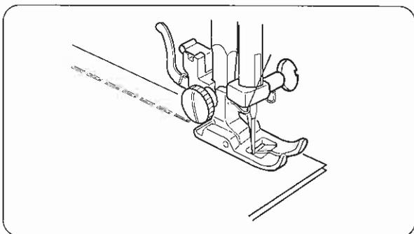
The stitch is sewn with two stitches forward and one stitch backward forming a seam that does not rip easily.
