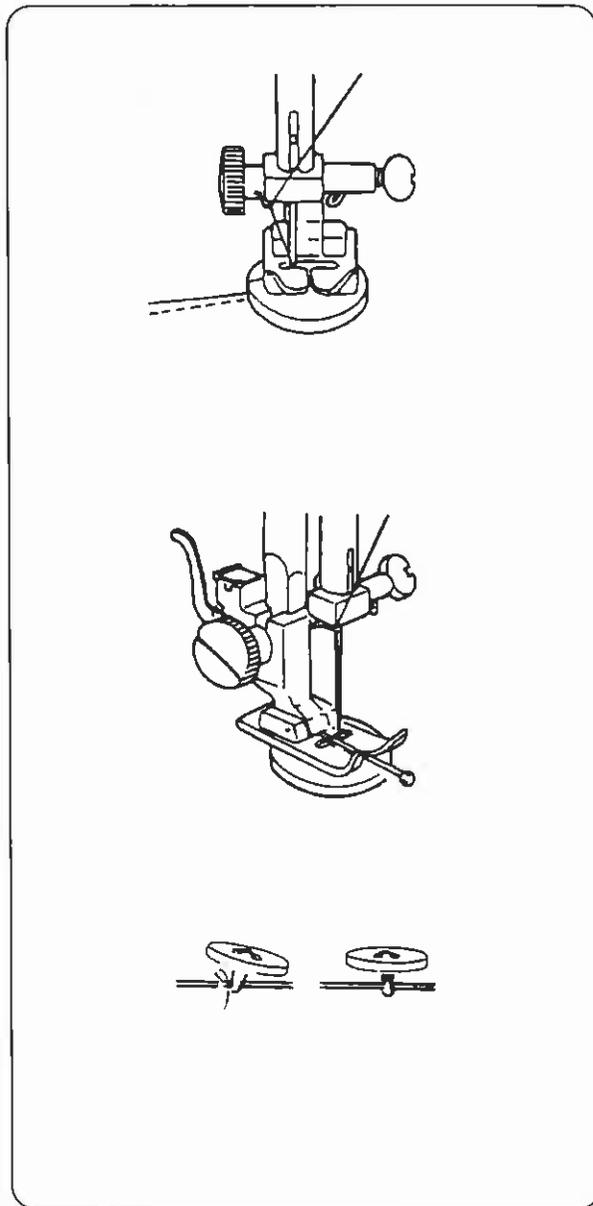
A pin can be placed on top of the foot to form a shank. Set the pattern selector at " B ".
