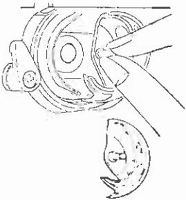
Open the hook race ring holders and remove the hook race ring.
