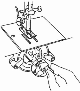
When inserting the bobbin case, place the horn into the recess of the hook race.
