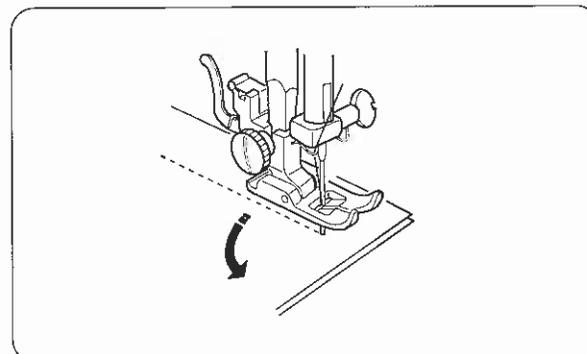
Raise the presser foot and position the fabric next to a stitching guide line on the needle plate. Lower the needle into the fabric. Lower the presser foot and smooth the threads toward the back. Depress the foot control. Gently guide the fabric along the guide line letting the fabric feed by itself.
