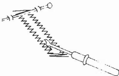
Set the pattern selector dial at “  $\frac{4}{2}$  ”, sew 5 stitches of bartack and raise the needle from the fabric.
