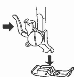
Press the lever on the back of the foot holder.
