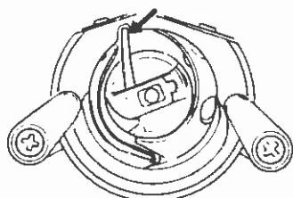
When inserting the bobbin case, place the horn into the recess of the hook race.
