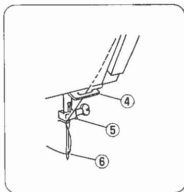
④ Then draw thread down and slip it into the lower thread guide.
