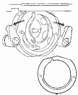
Open the hook race ring holders and remove the hook race ring.
