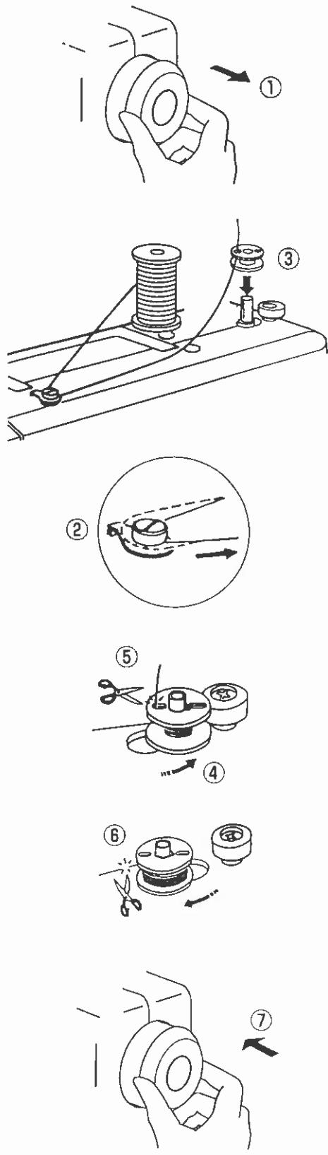
① Pull the handwheel out.
