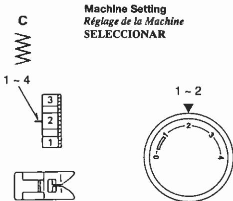
This type of stitch is used on the seam allowance to prevent fabrics from fraying at raw edges.
