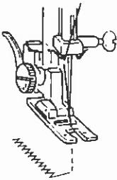
Set the pattern selector dial at " **4** ", sew 5 stitches of bartack and raise the needle from the fabric.
