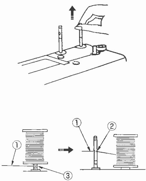
The spool pins are used for holding the spool of thread in order to feed thread to the machine.
