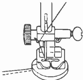
A pin can be placed on top of the foot to form a shank.
