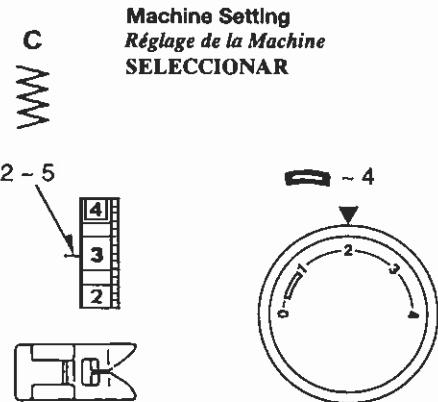
Simple zigzag stitching is widely used for overcasting, sewing on buttons, etc.
