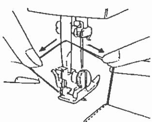
For fastening the ends of seams, press the reverse stitch button and sew several reverse stitches.
