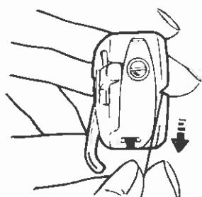
② Pull the thread into the bobbin case slot.
