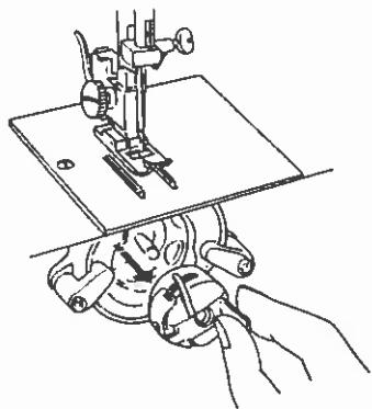
Raise the needle by turning the balance wheel toward you.
