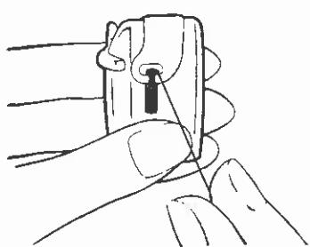
③ Draw the thread under the tension spring and into the delivery eye.
